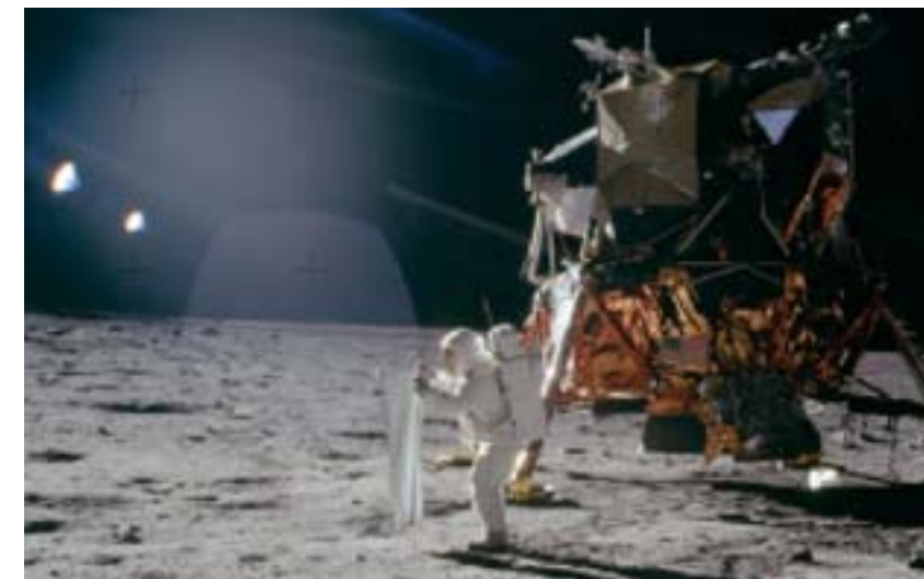
Figure 3: The US astronaut Edwin E. Aldrin unfurling the Solar Wind Composition (SWC) experiment of Johannes Geiss in the Mare Tranquilitatis on the Moon on 20 July 1969. This experiment was the first attempt to quantitatively analyse the composition of the solar wind. (NASA Photo S11-40-5872)
