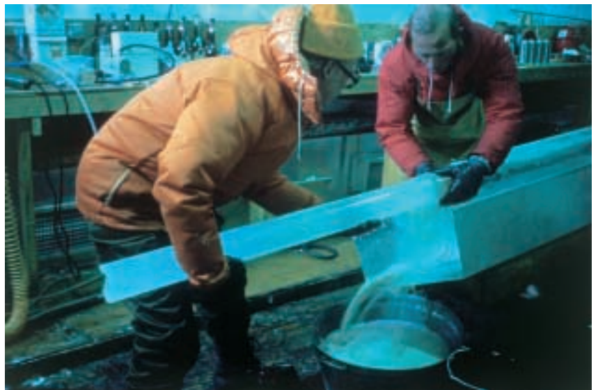
Figure 8 Deep-drilling (2,000 to 3,000 metres) is performed underground and takes about 2 to 3 years (Summer seasons). The drill is lowered into the borehole, drills a core of about 2,5 m length and is then brought up to the surface again. The picture shows how the ice-core is taken out of the drill. The liquid is used to prevent the borehole from closing.
