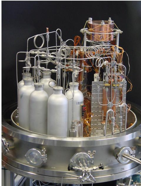
Figure 37.3: 4 K sorption-cooler prototype under development (Univ. Twente).
