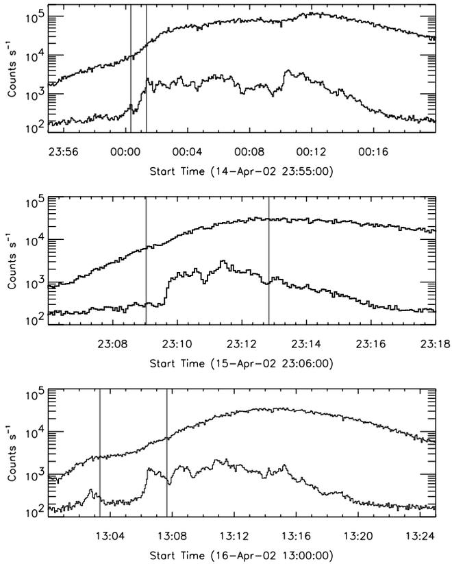
FIG. 1.—*RHESSI* light curves of the three flares, 2002 April 14–15 (*top*), 15 (*middle*), and 16 (*bottom*). The energy bands in each panel are 6–12 (*upper curve*) and 25–50 keV (*lower curve*). The solid lines in each panel mark the time range for the images in Figs. 2, 5, and 8. The time range was selected to show the *RHESSI* images with the coronal source above the flare loop.
