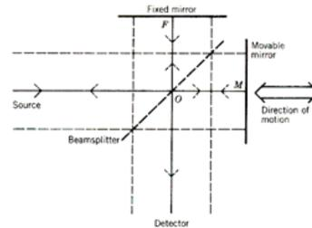
Schematic representation of a Michelson interferometer. The median ray is shown by the solid line, and the extremes of the collimated beam are shown by the broken lines.
