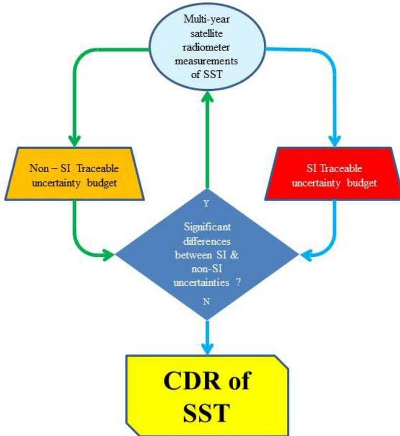
Figure 3. Simplified schematic for the generation of SST CDRs
