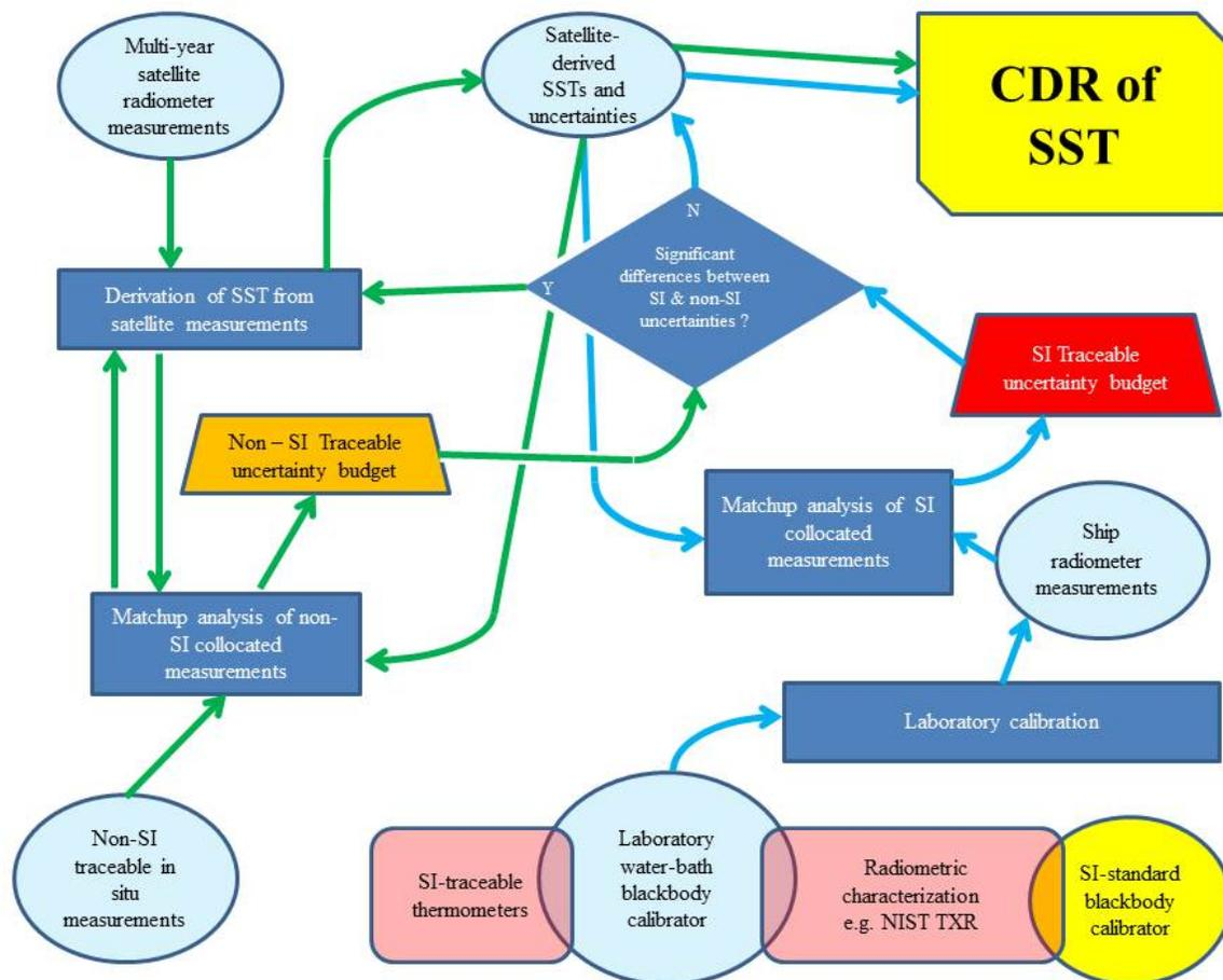
Figure 2. More complete form of the schematic for generating SST CDRs from satellite and in situ data.
