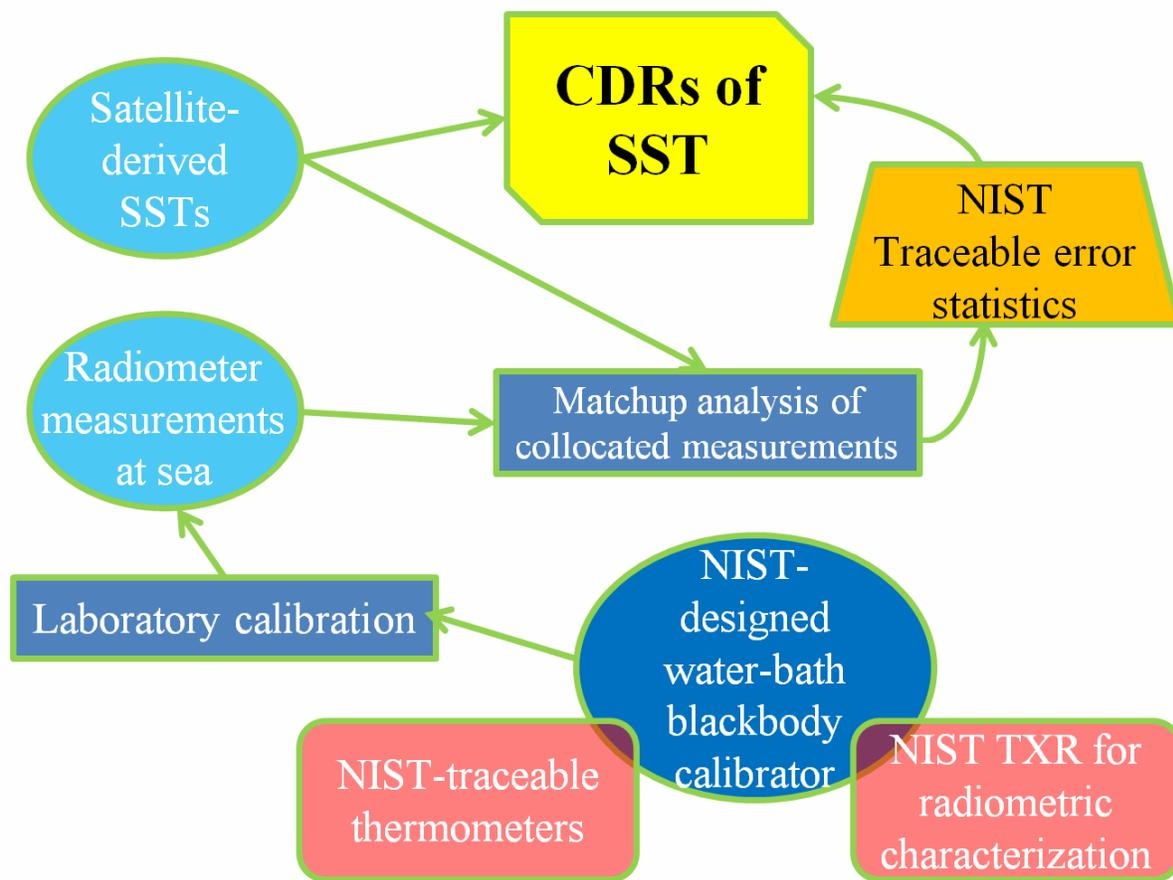
Figure 1 Schematic flow diagram for the generation of satellite-derived SST CDRs. From Minnett and Corlett, 2012.
