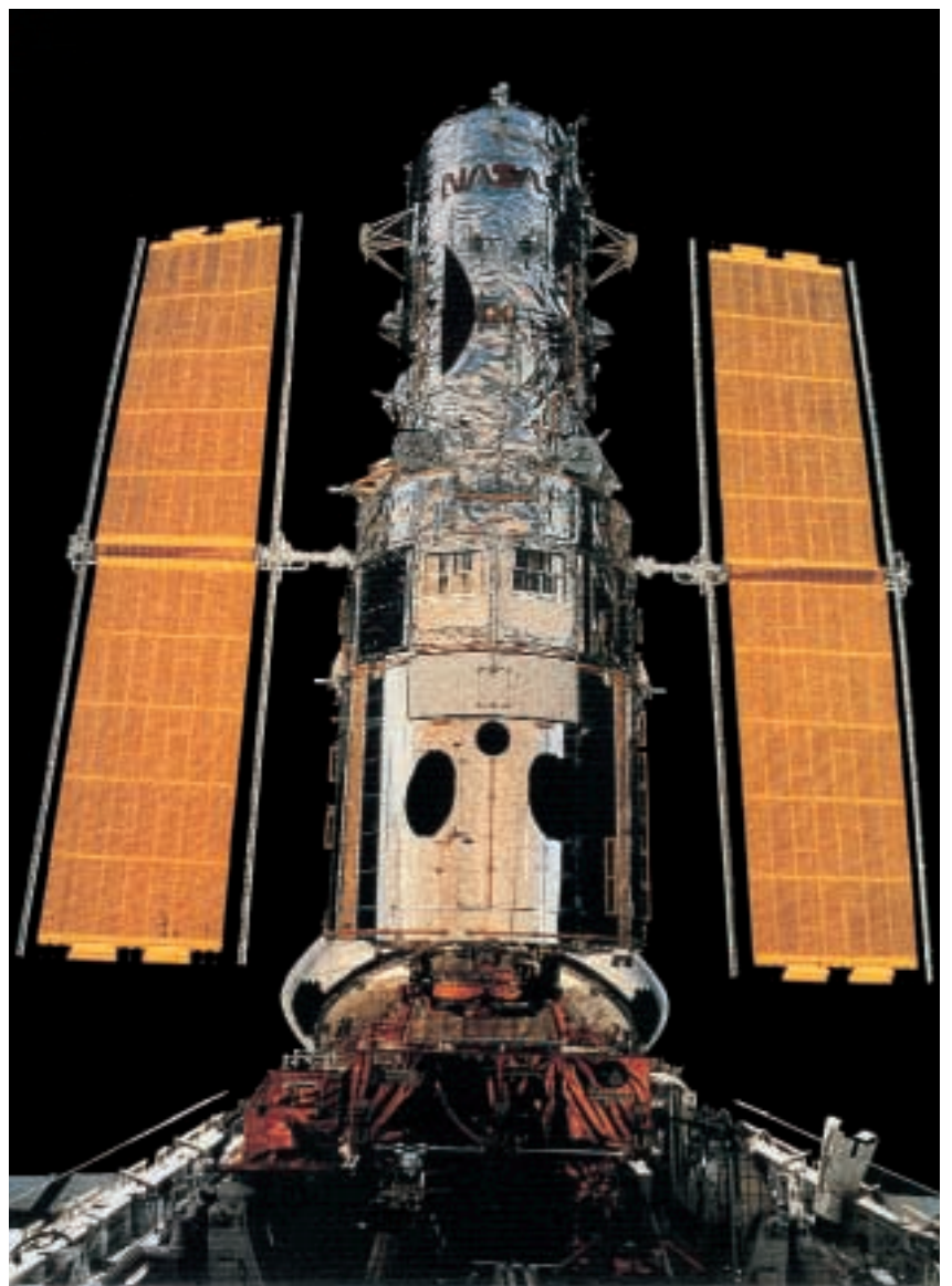
Figure 4. The Hubble Space Telescope has a mirror of “only” 2.5 m diameter, but since it orbits the Earth above the atmosphere it provides exceptionally sharp images. It has greatly helped to determine galaxy distances and hence to determine the expansion age of the Universe. The telescope was built and is operated by NASA with a 15% share of the European Space Agency (ESA). The telescope is here docked to the Space Shuttle during a repair mission involving the Swiss astronaut Claude Nicollier.
