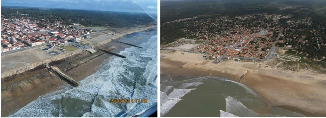
Figure 2: example of impacts of the interannual variability on coastal sediment availability in Montalivet (South-western France): left: situation after the exceptional storm season of 2013/2014; right: situation after the exceptional calm winter of 2014/2015. Exceptionally large differences in intertidal beach levels are obvious when comparing the two photos (source: Aquitaine Coastal Observatory/ONF/ULM Sud-Bassin)
