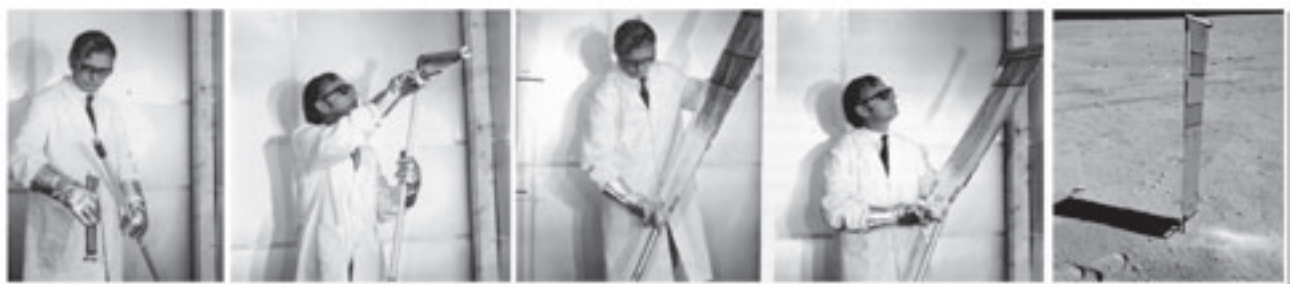
Fig. 13: The sequence of images show Johannes Geiss testing deployment and retrieval of the SWC foil in the thermal chamber at 80°C of Contraves Ltd. in Zurich, while the right image shows the SWC deployed on the lunar surface.
