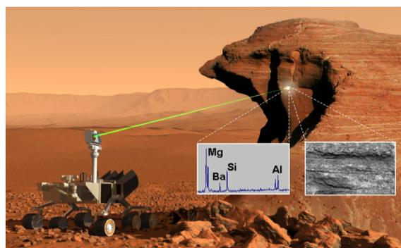
Figure 1: *Operational principle of ChemCam/LIBS on Mars (Credit CNES/NASA).*
