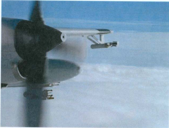
Counter flow virtual impactor mounted on a NCAR C130 wing
