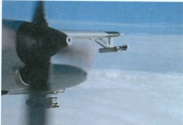
Counter flow virtual impactor mounted on plane wing
