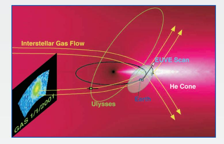
*Interstellar He distribution (color coded), as modeled by* J. Raymond, based on a hot model of the gas; typical location of Ulysses during the neutral He observations together with a sample of a sky image of the He flow; and a scan geometry for the He I 584 Å line glow through the focusing cone with EUVE from an October location.
