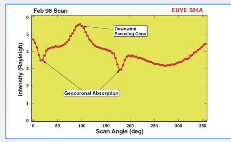
*The flux increase in the center represents the cone. The second* increase reflects the Earth's exospheric glow. The two dips are caused by resonant absorption of the He line by the exosphere in the directions where the velocity of the interstellar gas relative to the Earth is zero. The exact location of these features are used to deduce the He flow velocity.
