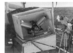
FIG. 2. The Atmospheric Emitted Radiance Interferometer aboard the Pelican .
