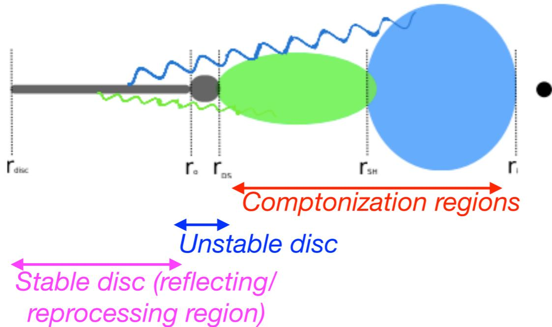
Disc truncated at  $\sim 20 r_g$  at the end of the transition from the soft to the hard state
