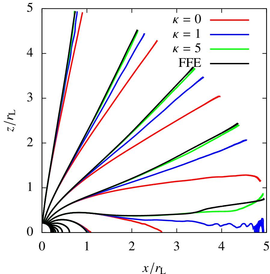
Figure 1: Magnetic field lines for the force-free magnetosphere in black solid lines, and radiative magnetosphere with  $\kappa \in \{0, 1, 5\}$  in respectively red, blue and green solid lines as shown in the legend.
