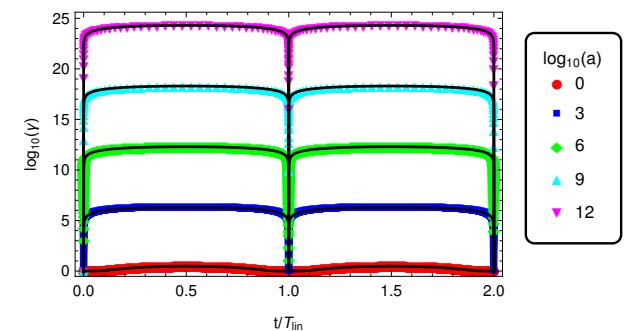
Figure 15: Lorentz factor of an electron for  $a = 10^i$  with  $i \in \{0, 3, 6, 9, 12, 15\}$ .
