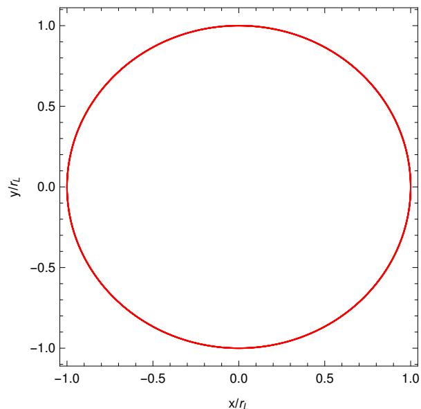
Figure 11: Gyromotion of an electron in the electric drift frame with  $\Gamma_E = 10^3$  and  $\gamma = 10^{10}$ . The Larmor radius is  $R_L = 10^{10}$ .
