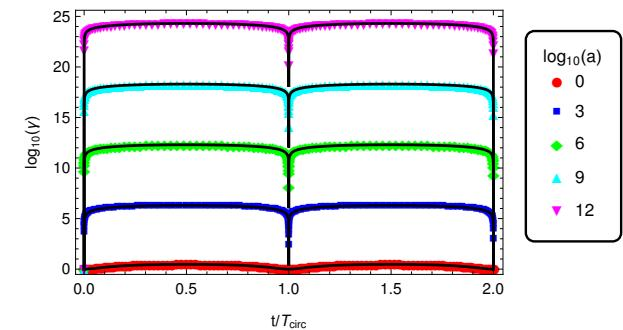
Figure 16: Lorentz factor of an electron for  $a = 10^i$  with  $i \in \{0, 3, 6, 9, 12, 15\}$ .
