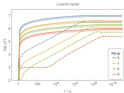
Fig. – Evolution of the Lorentz factor for a linearly polarized wave ( $\alpha = 0.5$ ) with  $a = 10^9$ , initial Lorentz factor  $\log \gamma_0 = \{0, 1, 2, 3\}$  and varying initial phases,  $\xi_0 = 0$  in dashed lines,  $\xi_0 = \pi/4$  in dotted lines and  $\xi_0 = \pi/2$  in solid lines.
