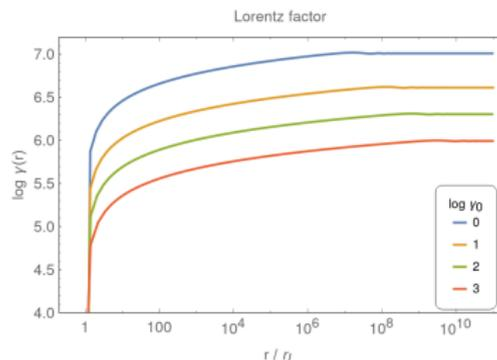
Fig. – Evolution of the Lorentz factor for a circularly polarized wave with  $a = 10^9$ , initial Lorentz factor  $\log \gamma_0 = \{0, 1, 2, 3\}$ . The curves are insensitive to the initial phase  $\xi_0$ .
