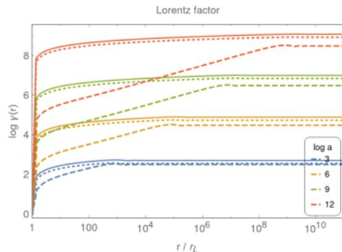
Fig. – Evolution of the Lorentz factor for a circularly, elliptically and linearly polarized wave respectively in solid, dotted and dashed line.
