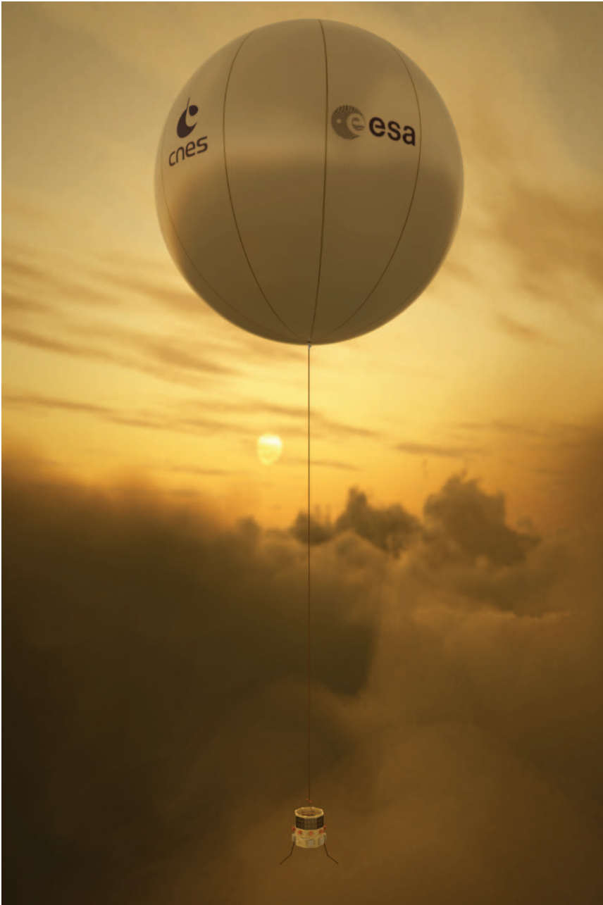
Figure 9.4: An artist's impression of the European Venus Explorer, EVE. The helium filled super pressure balloon/gondola combination will float at 55 km altitude and will make at least one full revolution around the planet during its minimum lifetime of ten days. Courtesy of T. Balint, JPL/Univ. Paris-Sud/Univ. Oxford
