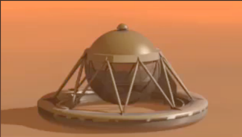
Artist's concept of Venus flagship lander on surface (pressure vessel can rotate for drill placement and image panoramas) Lander mass = 686 kg (x2)
