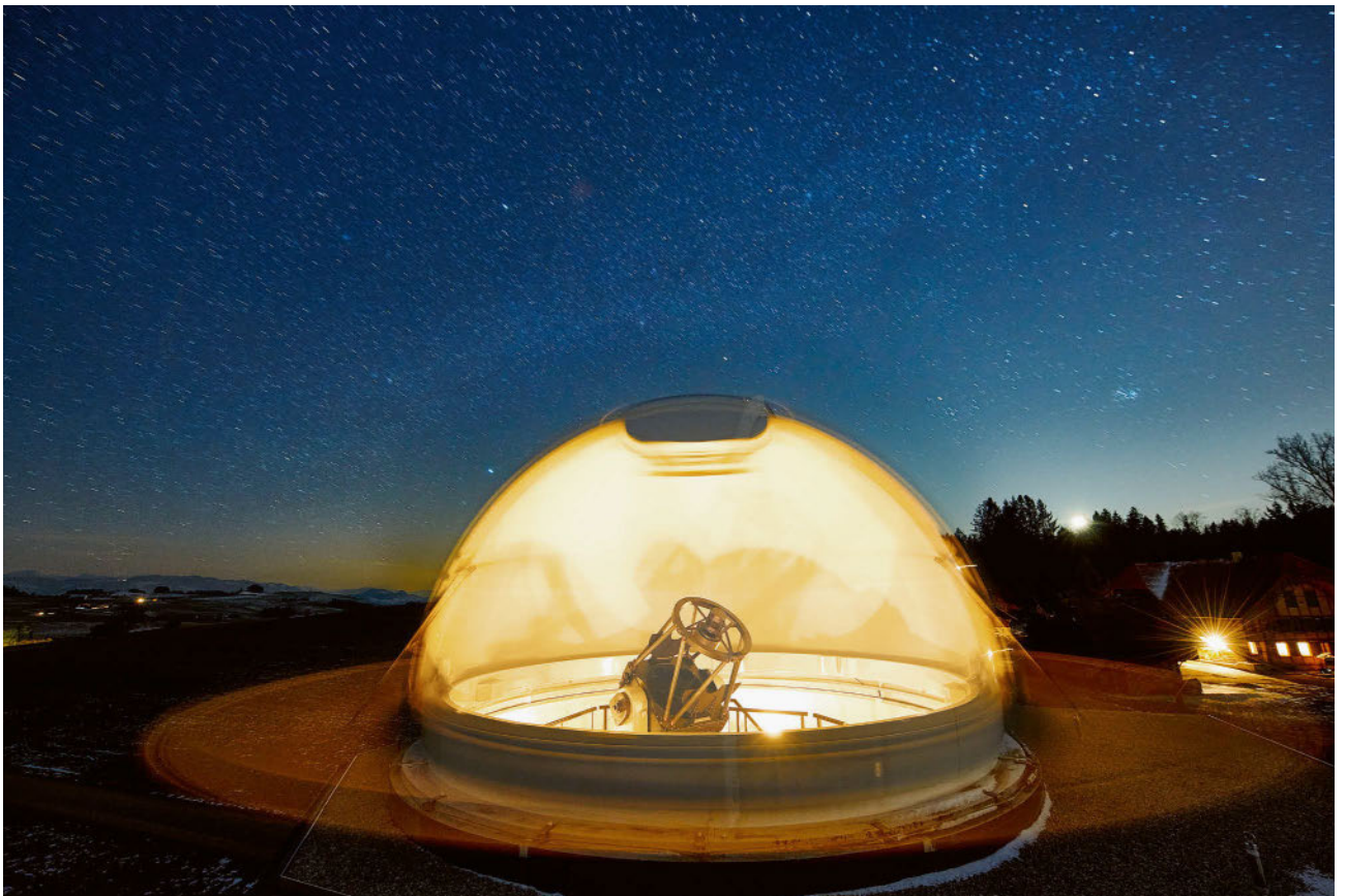
Figure 7: 0.8m Zimmerwald Multiple Applications Instrument ZimMAIN. Main applications are surveys for faint debris, and photometric and spectroscopic characterization of debris. (Credit: AIUB, Manu Friederich)
