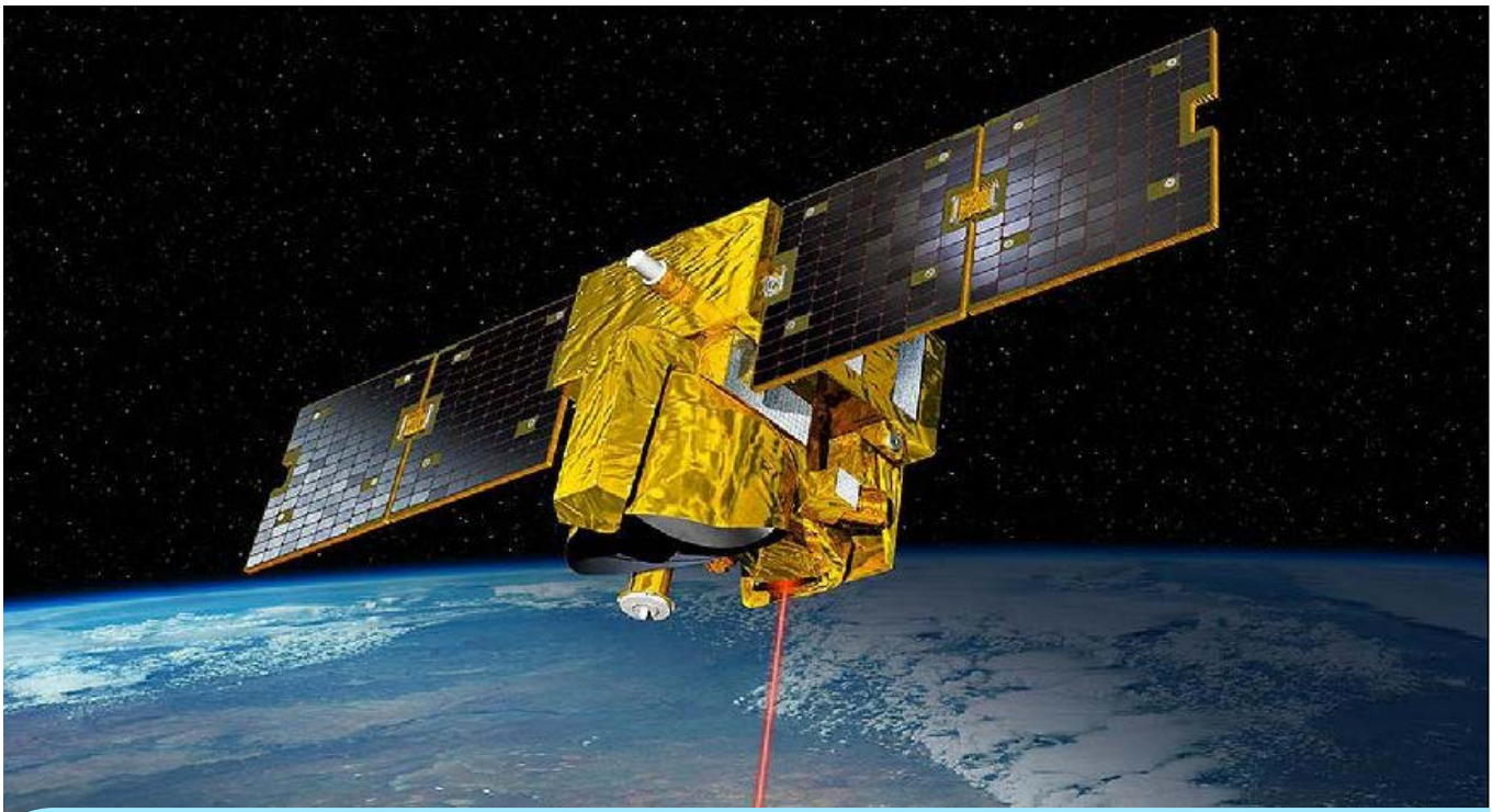
Figure 9. The CNES/DLR Methane Lidar Remote Sensing Mission (MERLIN) will use an active lidar system, at 1.65\mu\text{m} to retrieve column concentrations of methane. The active system will enable retrievals at nighttime and when the sun angles are low at high-latitudes. Figure by CNES/DLR.
