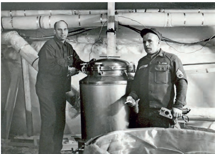
Fig. 73: Working in the ice tunnel of the US Army camp Tuto near Thule (now Qaanaaq) in Greenland. The vessel was used for the extraction of \text{CO}_2 from ice in order to determine the ^{14}\text{C} fraction (1965). (Credit: OCCR)
