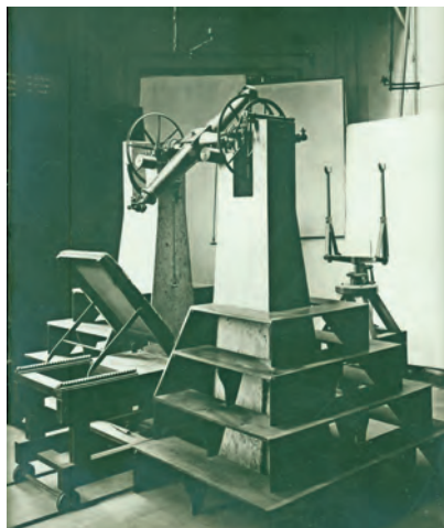
Fig. 25: The two pillar mount of the meridian circle by Ertel in the meridian hall of the Telluric Observatory in 1878. (Credit: AIUB)
