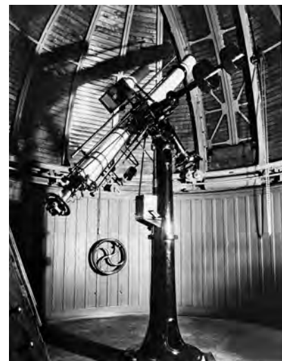
Fig. 43: The 175 mm refractor made by Merz in Munich in its dome at the Astronomical Institute. (Credit: AIUB)
