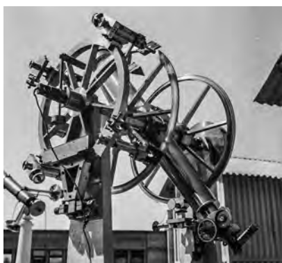
Fig. 44: The meridian circle made by Lerebours & Secrétan in Paris used at the Astronomical Institute for the observation of stellar occultations by the Moon. (Credit: StABE, FN Tschirren N 11.69, 8)
