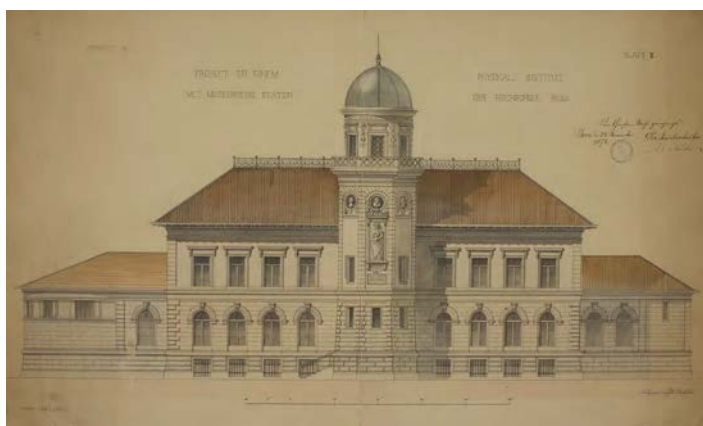
Fig. 22: Plan of the front side of the Telluric Observatory or Physics Institute, dated 25 November, 1875. Note that there were slight differences between this plan and the realized building, e. g., the extension on the right hand side of the main building does not correspond to the meridian hall as displayed on the photograph of Figure 23. (Credit: StABE, AA III 907, 1)
