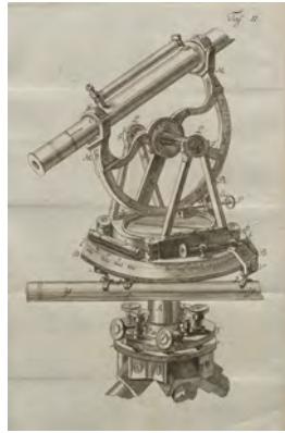
Fig. 4: Theodolite used by Tralles for measuring the mountains of the canton of Bern. (Credit: UB Bern, MUE H I 147)
