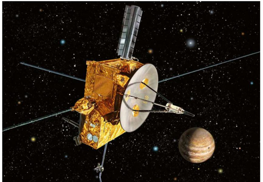
**Figure 2:** Ulysses, artist’s view. On the right and left diagonal, the radio plasma antennae can be seen, downwards pointing is the magnetometer boom, on the front the high-gain antenna. (Source: ESA/NASA, Public domain, via Wikimedia Commons).
